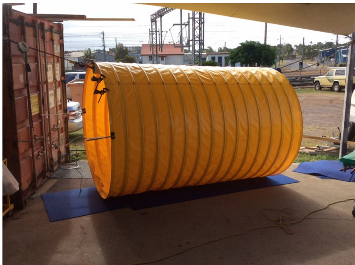
Ship Loader Dust Chute
